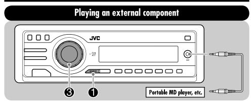
You can connect an external component to the LINE IN plug on the rear, and another to the AUX (auxiliary) input jack on the control panel.
